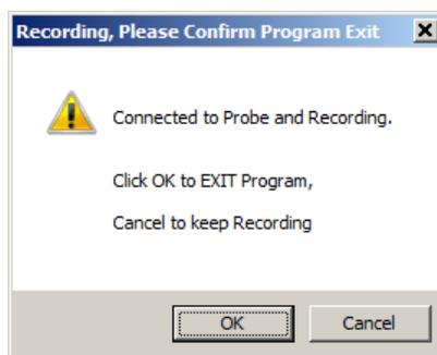
**Figure 4.** Warning dialogue to protect against accidental closure of the GUI during data acquisition.
